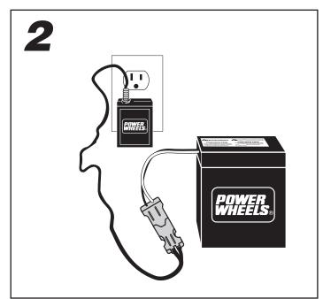
• Plug the charger into a standard 120 volt wall outlet. **Note:** If power flow to the wall outlet is controlled by a switch, make sure the switch is "ON".
